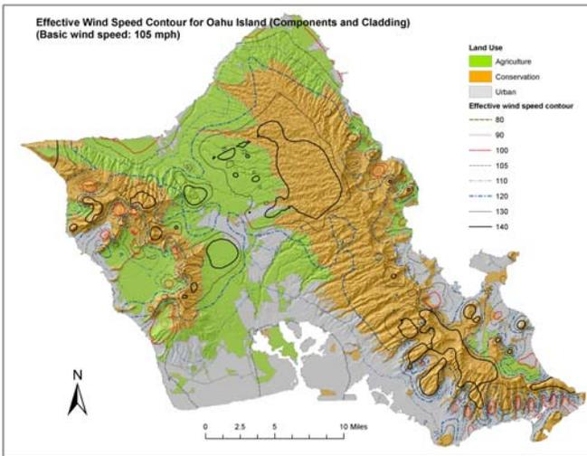
Figure 5: Effective Velocity  $V_{effective}$  Map for Oahu
