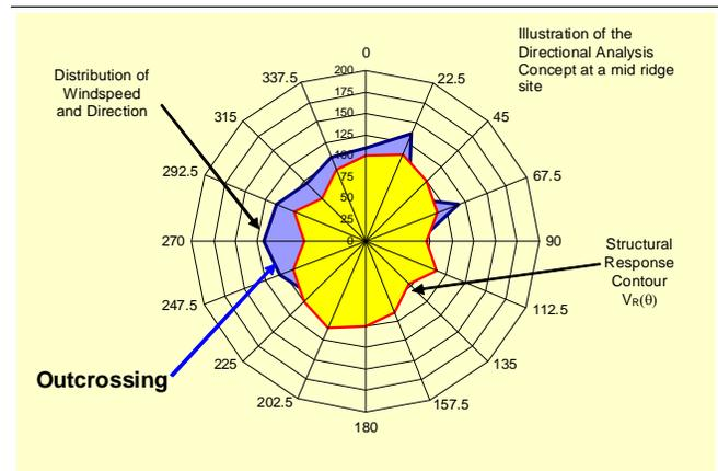
**Figure 3: Illustration of a Structural Response Function and Wind Speed Variation by Wind Direction**
